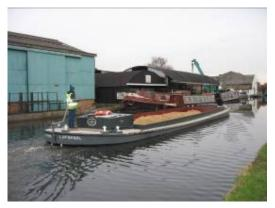
With the opening of two waterside sand and gravel facilities in west London, construction and development customers have been supplied with aggregate directly by barge. Motor barges can carry approx. 70 tonnes of aggregate and deliver to sites in west and central London within a few hours. On narrow canals deliveries by pairs of narrowboats are equally flexible.
