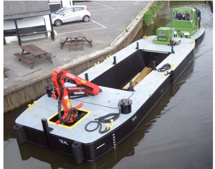
Hold Sized to Prevent Overloading
