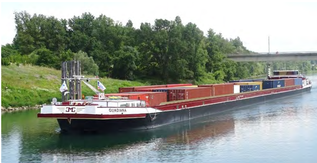
Motor container barge Guadiana, 135m x 11.45m, 3979t below Vienne on the river Rhône (R Rhone)
