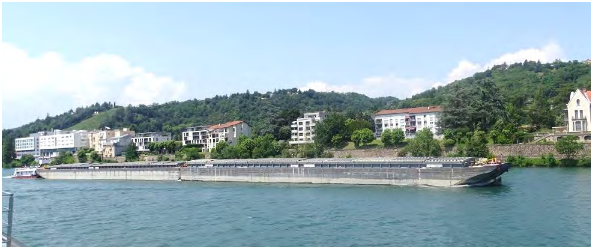
Two 82m x 11.4m pans 2710t each, with push tug below Vienne (R Horne)
