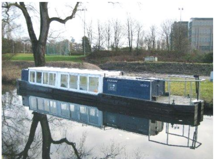
Science Daily says (drawing on material from the The converted hydrogen-fueled barge Ross Barlow with the EMPA-developed hydride storage tank. (EMPA).
