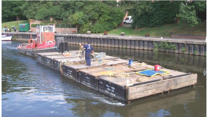
Alan Oliver's tug Exeter and uniflote dredging platforms going up to Hume lock in preparation for the dredging (L Reid)
