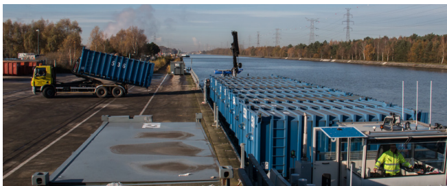
Roll-off containers being loaded onto a flat bed barge in Belgium
