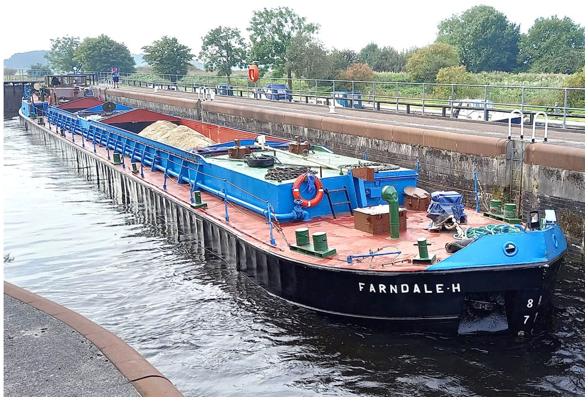
500-tonne capacity Branford Barge Owners' Farndale penning through Whitley lock with marine dredged aggregate for Leeds (A. Horn)
